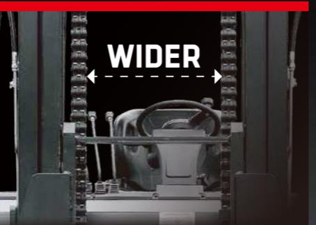
► The new design mast provides broad forward visibility due to outside located hydraulic pipes of fork positioner.
