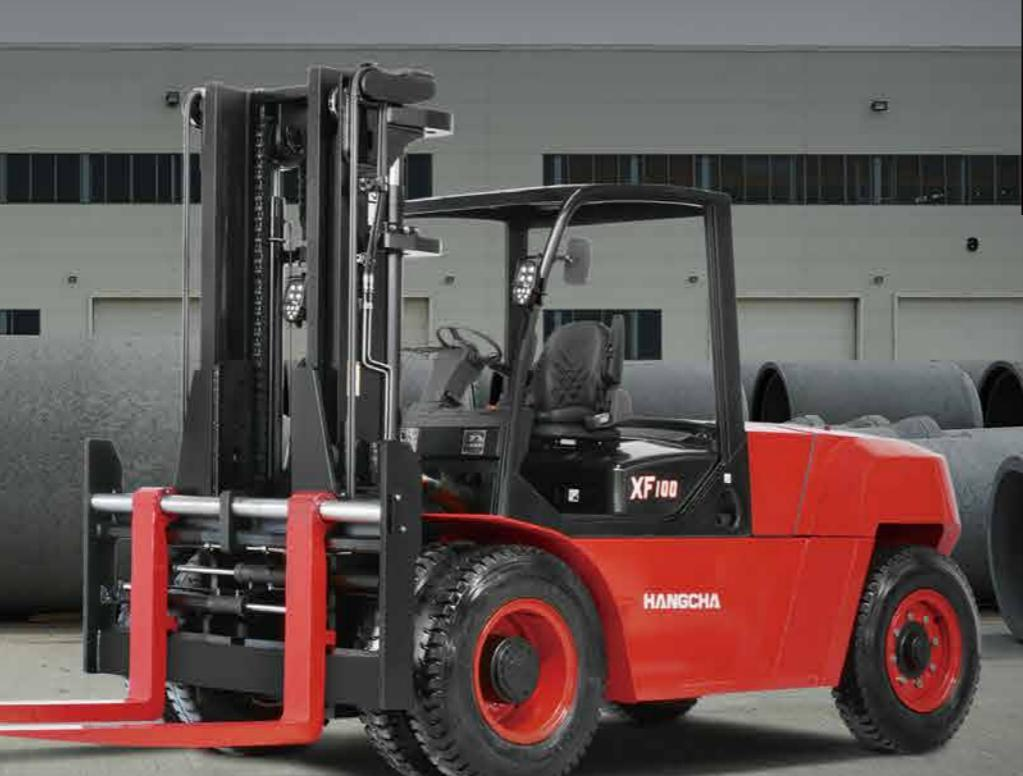
► The optional Electro-hydraulic proportional control system contributes more sensitive and precise load handling. The easy-to-operate levers provide total load handling operation. An armrest is provided to reduce fatigue.
